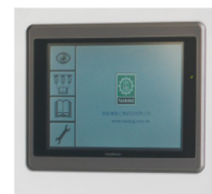
人機控制面板 (多錠共用一個設定面板) One computer terminal (central control panel for multi-spindles)
