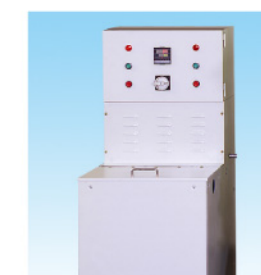
循環式加熱油箱 Hot circulating oiling tank
