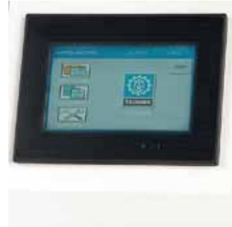
人機控制面板 (多錠共用一個設定面板) One computer terminal (central control panel) for multi-spindles.
