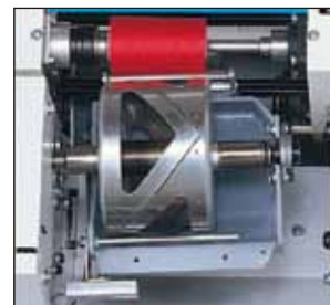
滾筒式導線裝置 Drum thread-guiding system
