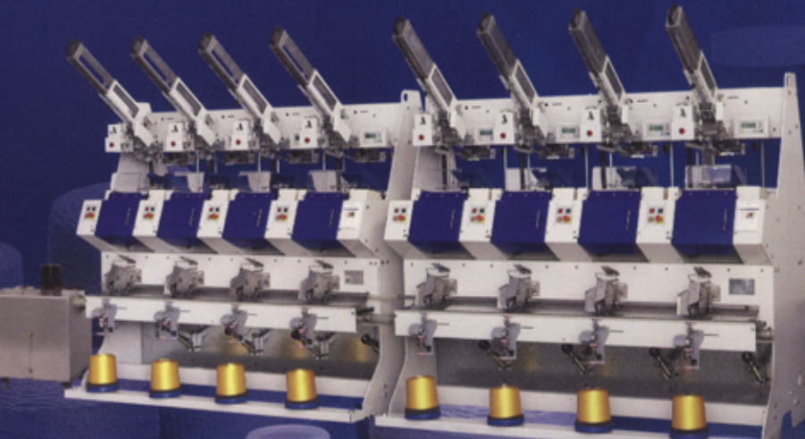
TN-35A全自動高速繞線機-H型管 Automatic High Speed Cross Cone Winder(Spool Type)
